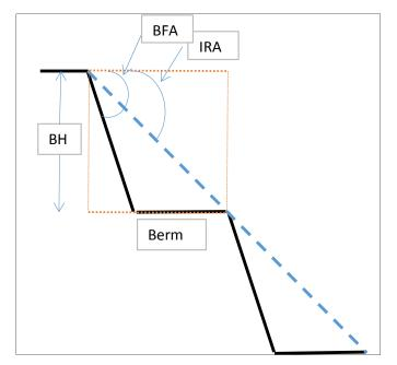
Figure 16-3: Slope Parameters
