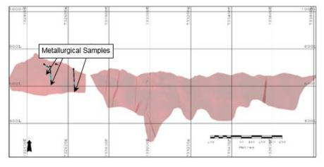
Figure 13-1: A Vulcan<sup>®</sup> Snapshot (looking north) of the Moss Deposit Showing the Positions of the Composites, McClelland Laboratories 2015 Test Program, Moss Mine Project
