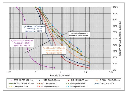
Figure 13-4: A Scatter Plot of Particle Size Distributions for 6.35 mm (¼") Composites Tested During Various Metallurgical Programs, Moss Mine Project
