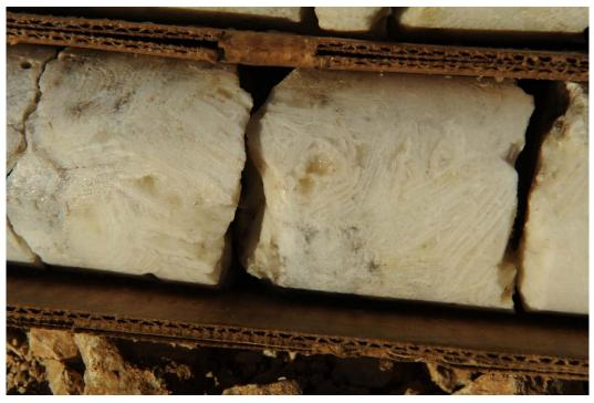
Figure 8-1: Bladed Calcite Partially Replaced by Quartz - Evidence of Boiling (AR 165 213 ft)
