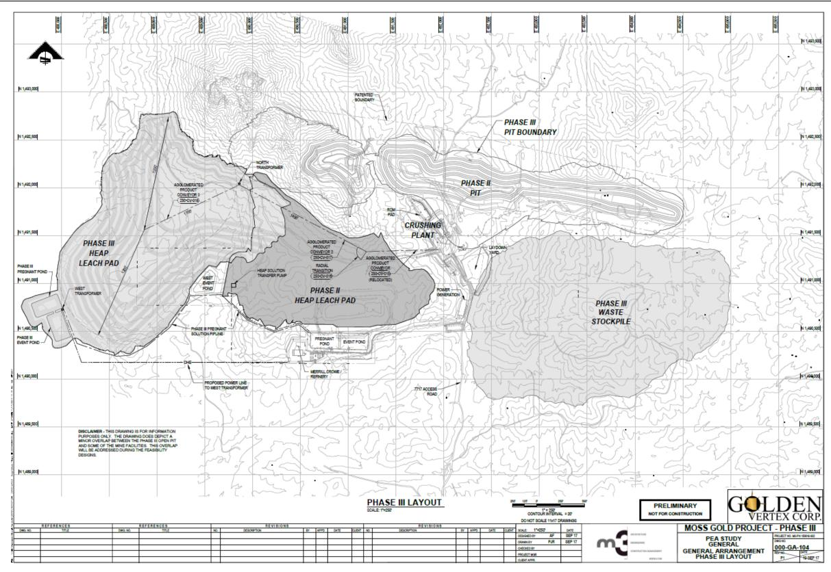
Figure 17-2: General Arrangement Site Plan
